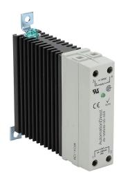
AutomationDirect solid state relay, 35mm DIN rail mount, fingersafe, 4-32 VDC input voltage, SPST, (1) N.O. SCR, 30A contact rating, 24-280 VAC load voltage, random cross, screw terminal(s), LED indicator(s).
