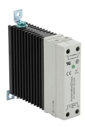
AutomationDirect solid state relay, 35mm DIN rail mount, fingersafe, 90-280 VAC input voltage, SPST, (1) N.O. SCR, 30A contact rating, 24-280 VAC load voltage, random cross, screw terminal(s), LED indicator(s).
