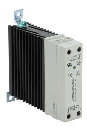
AutomationDirect solid state relay, 35mm DIN rail mount, fingersafe, 4-32 VDC input voltage, SPST, (1) N.O. SCR, 10A contact rating, 24-280 VAC load voltage, random cross, screw terminal(s), LED indicator(s).
