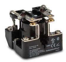
AutomationDirect power relay, panel mount, open, 12 VDC coil voltage, DPST, (2) N.O., 40A contact rating, screw terminal(s).
