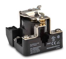
AutomationDirect power relay, panel mount, open, 12 VDC coil voltage, SPDT, (1) N.O., (1) N.C., 40A contact rating, screw terminal(s).
