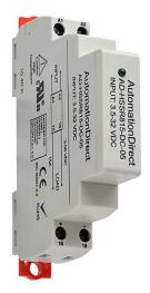
AutomationDirect solid state relay, 35mm DIN rail mount, fingersafe, 3.5-32 VDC input voltage, SPST, (1) N.O. MOSFET, 15A contact rating, 3-50 VDC load voltage, DC switching, screw terminal(s), LED indicator(s), hazardous location certified.
