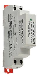
AutomationDirect solid state relay, 35mm DIN rail mount, fingersafe, 3-32 VDC input voltage, SPST, (1) N.O. SCR, 10A contact rating, 48-600 VAC load voltage, zero cross, screw terminal(s), LED indicator(s), hazardous location certified.
