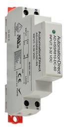
AutomationDirect solid state relay, 35mm DIN rail mount, fingersafe, 3-32 VDC input voltage, SPST, (1) N.O. SCR, 10A contact rating, 48-600 VAC load voltage, zero cross, screw terminal(s), LED indicator(s), hazardous location certified.
