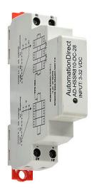
AutomationDirect solid state relay, 35mm DIN rail mount, fingersafe, 3-32 VDC input voltage, SPST, (1) N.O. SCR, 10A contact rating, 24-280 VAC load voltage, zero cross, screw terminal(s), LED indicator(s), hazardous location certified.
