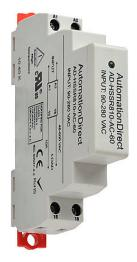
AutomationDirect solid state relay, 35mm DIN rail mount, fingersafe, 90-280 VAC input voltage, SPST, (1) N.O. SCR, 10A contact rating, 48-600 VAC load voltage, zero cross, screw terminal(s), LED indicator(s), hazardous location certified.
