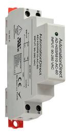
AutomationDirect solid state relay, 35mm DIN rail mount, fingersafe, 90-280 VAC input voltage, SPST, (1) N.O. SCR, 10A contact rating, 48-600 VAC load voltage, zero cross, screw terminal(s), LED indicator(s), hazardous location certified.
