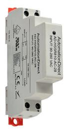
AutomationDirect solid state relay, 35mm DIN rail mount, fingersafe, 90-280 VAC input voltage, SPST, (1) N.O. SCR, 10A contact rating, 24-280 VAC load voltage, zero cross, screw terminal(s), LED indicator(s), hazardous location certified.
