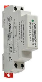
AutomationDirect solid state relay, 35mm DIN rail mount, fingersafe, 3.5-32 VDC input voltage, SPST, (1) N.O. MOSFET, 8A contact rating, 3-150 VDC load voltage, DC switching, screw terminal(s), LED indicator(s), hazardous location certified.
