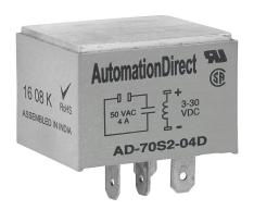
AutomationDirect solid state relay, socket mount, encapsulated, 3-30 VDC input voltage, SPST, (1) N.O. TRIAC, 4A contact rating, 8-50 VAC load voltage, zero cross, 4-pin. Requires 782-2C-SKT mounting socket.
