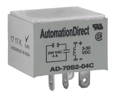
AutomationDirect solid state relay, socket mount, encapsulated, 3-30 VDC input voltage, SPST, (1) N.O. TRIAC, 4A contact rating, 24-280 VAC load voltage, zero cross, 4-pin. Requires 782-2C-SKT mounting socket.
