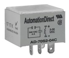
AutomationDirect solid state relay, socket mount, encapsulated, 3-30 VDC input voltage, SPST, (1) N.O. TRIAC, 4A contact rating, 24-280 VAC load voltage, zero cross, 4-pin. Requires 782-2C-SKT mounting socket.
