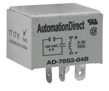
AutomationDirect solid state relay, socket mount, encapsulated, 3-30 VDC input voltage, SPST, (1) N.O. TRIAC, 4A contact rating, 24-140 VAC load voltage, zero cross, 4-pin. Requires 782-2C-SKT mounting socket.
