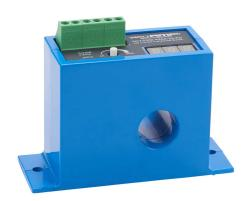
AcuAMP AC current transducer/switch, 1-phase, fixed core, 0-200A sensing range, 4-200A adjustable trip point, single-turn potentiometer with trip point display, 4-20 mA or solid state switch, N.O. output, 1A @ 240 VAC output rating.
