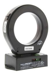
AcuAMP AC current transducer, 1-phase, fixed core, 0-1000, 0-1333, or 0-2000A selectable sensing range, True RMS, 4-20 mA output.
