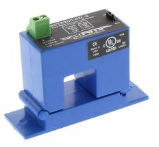
AcuAMP AC current transducer, 1-phase, split core, 0-100, 0-150, or 0-200A selectable sensing range, True RMS, 4-20 mA output.
