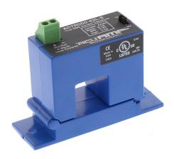
AcuAMP AC current transducer, 1-phase, split core, 0-10, 0-20, or 0-50A selectable sensing range, True RMS, 4-20 mA output.
