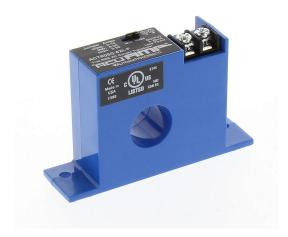
AcuAMP AC current transducer, 1-phase, fixed core, 0-10, 0-20, or 0-50A selectable sensing range, True RMS, 4-20 mA output.
