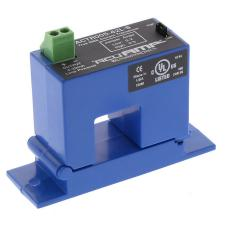
AcuAMP AC current transducer, 1-phase, split core, 0-2 or 0-5A selectable sensing range, True RMS, 4-20 mA output.
