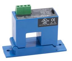
AcuAMP AC current transducer, 1-phase, split core, 0-10, 0-20, 0-50A selectable, with time integration sensing range, True RMS, 4-20 mA output.
