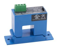
AcuAMP AC current transducer, 1-phase, split core, 0-10, 0-20, 0-50A selectable, with time integration sensing range, True RMS, 4-20mA output.
