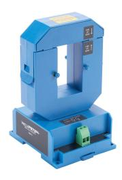
AcuAMP AC current transducer, 1-phase, split core, 0-400A sensing range, 4-20 mA output.
