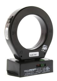
AcuAMP AC current transducer, 1-phase, fixed core, 0-1000, 0-1333, or 0-2000A selectable sensing range, 4-20 mA output.
