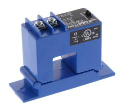
AcuAMP AC current transducer, 1-phase, split core, 0-100, 0-150, or 0-200A selectable sensing range, 4-20 mA output.
