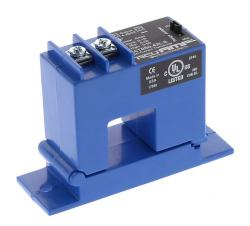
AcuAMP AC current transducer, 1-phase, split core, 0-10, 0-20, or 0-50A selectable sensing range, 4-20 mA output.
