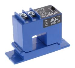
AcuAMP AC current transducer, 1-phase, split core, 0-10, 0-20, or 0-50A selectable sensing range, 0-10 VDC output.
