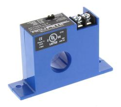
AcuAMP AC current transducer, 1-phase, fixed core, 0-10, 0-20, or 0-50A selectable sensing range, 0-10 VDC output.
