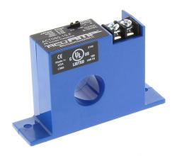
AcuAMP AC current transducer, 1-phase, fixed core, 0-10, 0-20, or 0-50A selectable sensing range, 0-10 VDC output.
