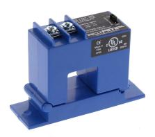
AcuAMP AC current transducer, 1-phase, split core, 0-2 or 0-5A selectable sensing range, 4-20 mA output.
