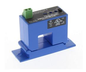
AcuAMP AC current switch, split core, 2-12, 12-55, or 55-200A selectable sensing range, 2-200A adjustable trip point, 4-turn potentiometer, solid state switch, N.C., adjustable time delay output, 0.2A @ 135 VAC/VDC output rating.
