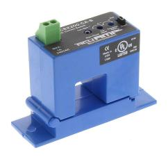
AcuAMP AC current switch, split core, 2-12, 12-55, or 55-200A selectable sensing range, 2-200A adjustable trip point, 4-turn potentiometer, solid state switch, N.C., adjustable time delay output, 1A @ 240 VAC output rating.
