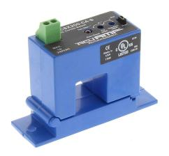
AcuAMP AC current switch, split core, 2-12, 12-55, or 55-200A selectable sensing range, 2-200A adjustable trip point, 4-turn potentiometer, solid state switch, N.C., adjustable time delay output, 1A @ 240 VAC output rating.
