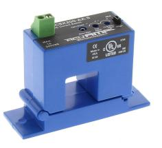
AcuAMP AC current switch, split core, 2-12, 12-55, or 55-200A selectable sensing range, 2-200A adjustable trip point, 4-turn potentiometer, solid state switch, N.O., adjustable time delay output, 1A @ 240 VAC output rating.
