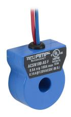
AcuAMP AC current switch, fixed core, 0-100A sensing range, 0.5A non-adjustable trip point, solid state switch, N.O. output, 0.15A @ 120 VAC/VDC output rating.
