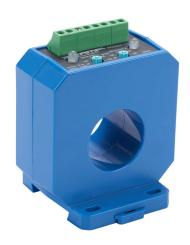
AcuAMP AC current switch, fixed core, 25-400A sensing range, (2) 25-400A adjustable trip point, (2) single-turn potentiometers, (2) SPDT relays output, 1A @ 120 VAC, 2A @ 30 VDC output rating.
