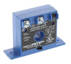
AcuAMP AC current switch, fixed core, 1-6, 6-40, or 40-175A selectable sensing range, 1-175A adjustable trip point, 4-turn potentiometer, solid state switch, N.C. output, 0.15A @ 30 VDC output rating.
