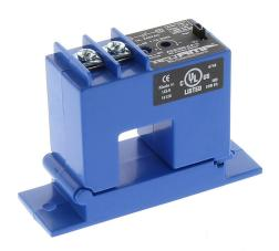
AcuAMP AC current switch, split core, 1.75-6, 6-40, or 40-200A selectable sensing range, 1.75-200A adjustable trip point, 4-turn potentiometer, solid state switch, N.C. output, 1A @ 240 VAC output rating.
