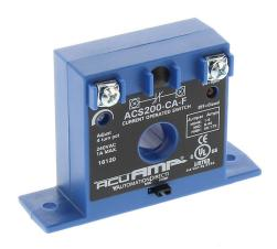
AcuAMP AC current switch, fixed core, 1-6, 6-40, or 40-175A selectable sensing range, 1-175A adjustable trip point, 4-turn potentiometer, solid state switch, N.C. output, 1A @ 240 VAC output rating.
