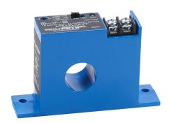
AcuAMP AC current switch, fixed core, 1-6, 6-40, or 40-175A selectable sensing range, 1-175A adjustable trip point, 15-turn potentiometer, solid state switch, N.C. output, 1A @ 240 VAC output rating.
