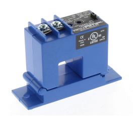
AcuAMP AC current switch, split core, 1.75-6, 6-40, or 40-200A selectable sensing range, 1.75-200A adjustable trip point, 4-turn potentiometer, solid state switch, N.O. output, 1A @ 240 VAC output rating.
