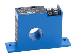
AcuAMP AC current switch, fixed core, 1-6, 6-40, or 40-175A selectable sensing range, 1-175A adjustable trip point, 15-turn potentiometer, solid state switch, N.O. output, 1A @ 240 VAC output rating.
