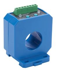
AcuAMP AC current switch, fixed core, 2-35A sensing range, (2) 2-35A adjustable trip point, (2) single-turn potentiometers, (2) SPDT relays output, 1A @ 120 VAC, 2A @ 30 VDC output rating.
