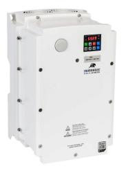
IronHorse ACN series AC general purpose drive, NEMA 4X, 460 VAC, 15hp with 3-phase input, 7-1/2hp with 1-phase input, SVC, V/Hz or torque mode, 4 frame, RS-485, integrated dynamic braking. Optional EtherNet/IP and Modbus TCP card available.
