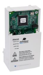
IronHorse ACN series communication module, EtherNet/IP and Modbus TCP, 1 port, (1) Ethernet (RJ45) and (1) RS-232 (RJ45) port(s). For use with IronHorse ACN series drives. Mounting hardware included.
