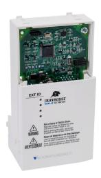
IronHorse ACN series relay/analog combo module, Analog Input: 2-channel, current/voltage, Analog Output: 1-channel, current/voltage, Discrete Input: 3-point, sinking/sourcing, Discrete Output: 2-point, relay, (2) Form C (SPDT) relays.
