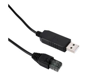
IronHorse programming/communication cable, 3.2ft/1m cable length, RS-232 (RJ45 8P8C) to USB A. Not compatible with Windows 11 software. Instead use USB-485M PC adapter.
