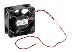
IronHorse ACG series main cooling fan, replacement,  $60 \times 60 \times 25$ mm, 24 VDC. For use with ACG series 2hp - 5hp AC drives.
