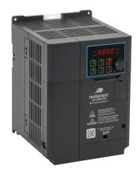
IronHorse ACG series AC general purpose drive, enclosed, 460 VAC, 5hp with 3-phase input, 2hp with 1-phase input, SVC or V/Hz mode, C frame, RS-485, Modbus, 100kA SCCR. Optional EtherNet/IP and Modbus TCP card available.
