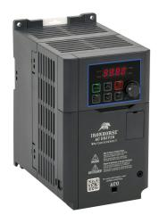
IronHorse ACG series AC general purpose drive, enclosed, 460 VAC, 2hp with 3-phase input, 1hp with 1-phase input, SVC or V/Hz mode, B frame, RS-485, Modbus, 100kA SCCR. Optional EtherNet/IP and Modbus TCP card available.
