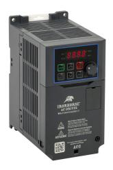
IronHorse ACG series AC general purpose drive, enclosed, 460 VAC, 1hp with 3-phase input, 1/2hp with 1-phase input, SVC or V/Hz mode, A frame, RS-485, Modbus, 100kA SCCR. Optional EtherNet/IP and Modbus TCP card available.
