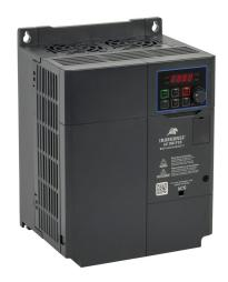
IronHorse ACG series AC general purpose drive, enclosed, 230 VAC, 7-1/2hp with 3-phase input, 3hp with 1-phase input, SVC or V/Hz mode, D frame, RS-485, Modbus, 100kA SCCR. Optional EtherNet/IP and Modbus TCP card available.
