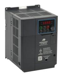
IronHorse ACG series AC general purpose drive, enclosed, 230 VAC, 5hp with 3-phase input, 2hp with 1-phase input, SVC or V/Hz mode, C frame, RS-485, Modbus, 100kA SCCR. Optional EtherNet/IP and Modbus TCP card available.
